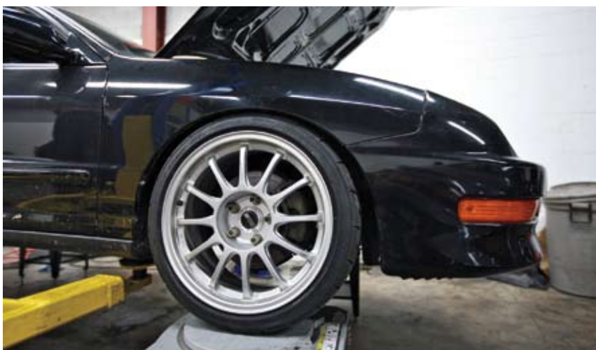
Sometimes you need a little persuasion to help make something fit. A metal bar worked wonders for rolling and pulling the fenders out to fit the wheels and tires.
