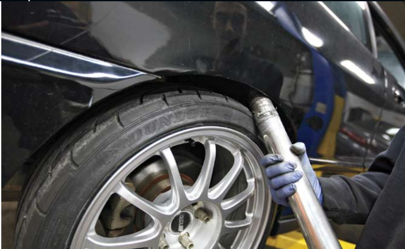
Sometimes you need a little persuasion to help make something fit. A metal bar worked wonders for rolling and pulling the fenders out to fit the wheels and tires.
