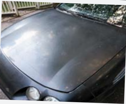
This hood is as faded as it comes. It's lost almost all of its clearcoat.
