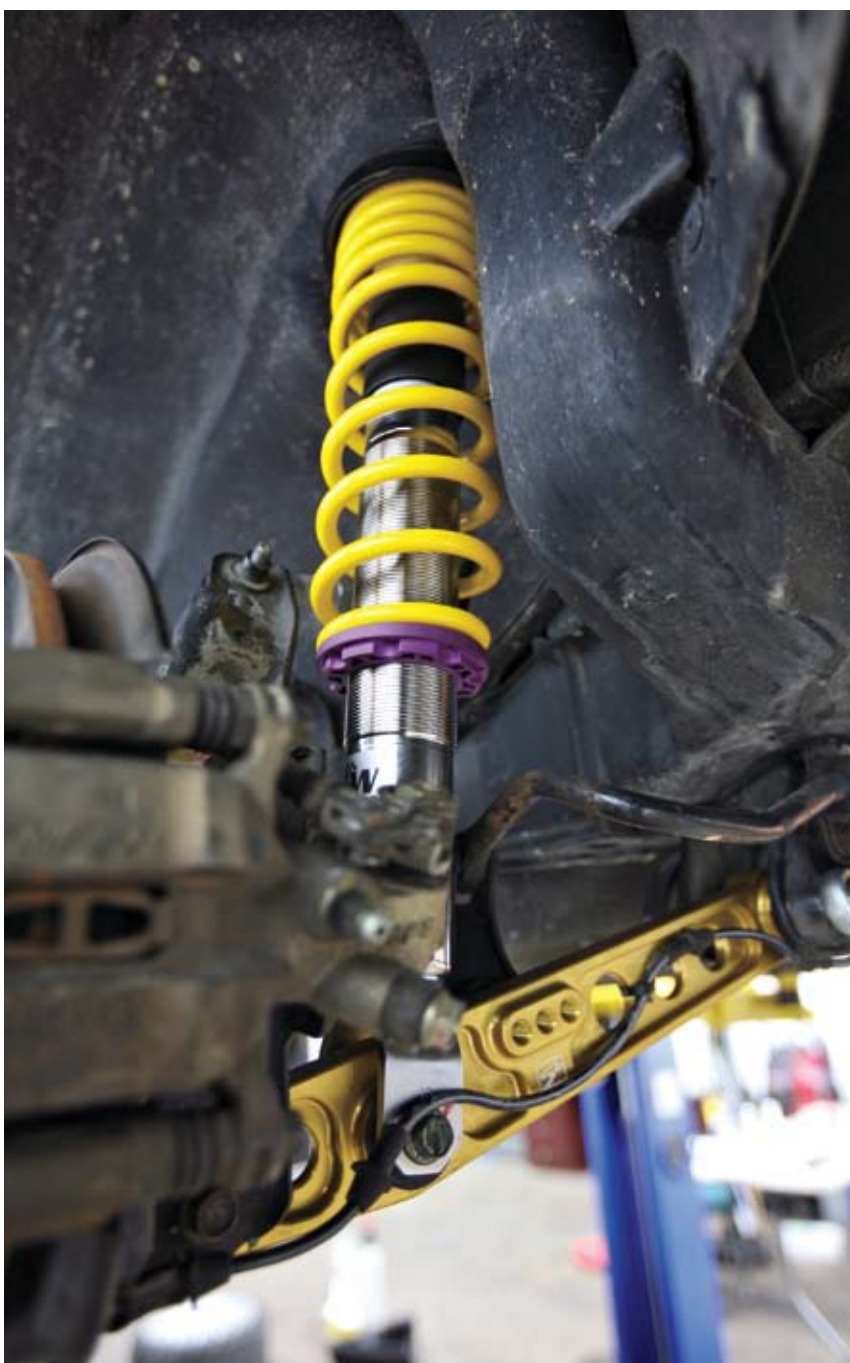
The KWs provide both compression and rebound adjustment, making them the ultimate tunable coilover.
