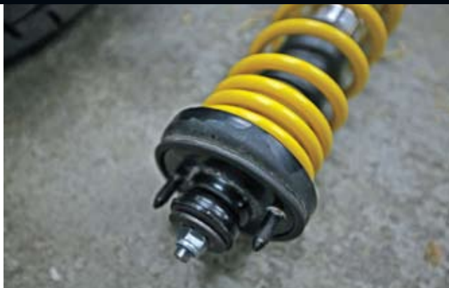
The stock top hats have to be installed onto the KW V3 coilovers. They will provide more comfort for the street over metal-type top hats.
