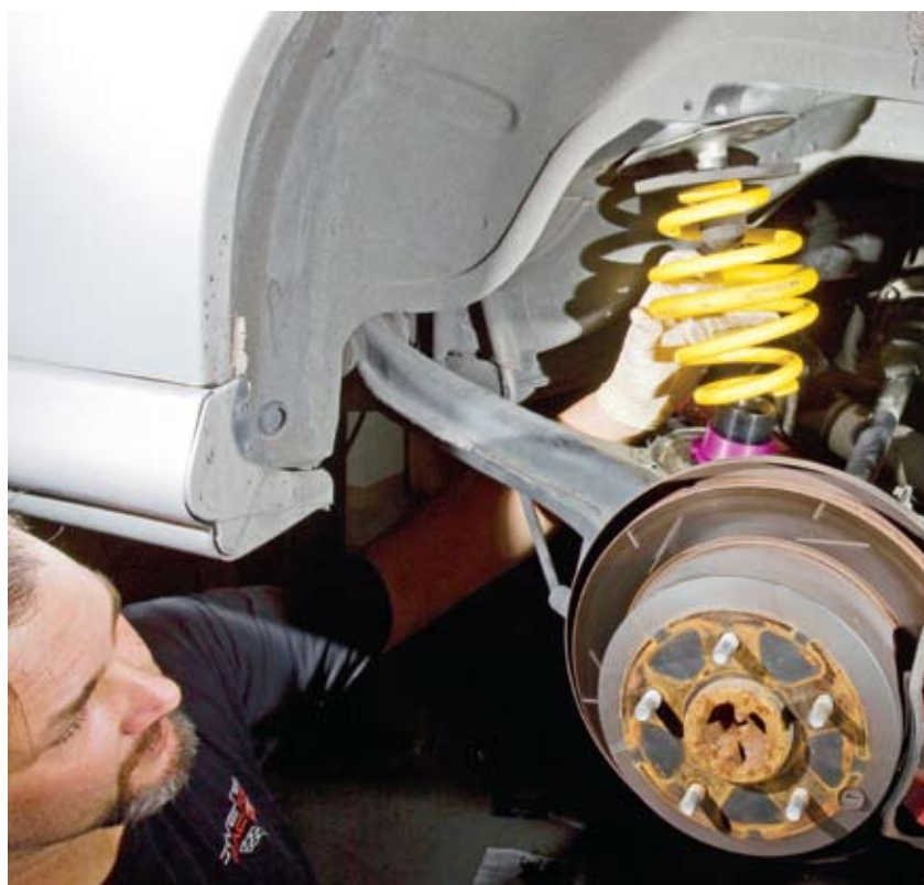
Greg Lovell installs the GTO's KW rear coil spring during our suspension install.
